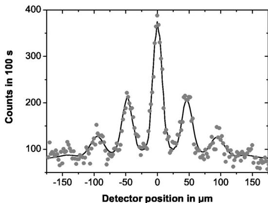
Fig. 7. Far-field diffraction of  $C_{60}$  using the slotted disk velocity selector. The mean velocity was  $\bar{v} = 117$  m/s, and the width was  $\Delta v/v \sim 17\%$ . Full circles represent the experimental data. The full line is a numerical model based on Kirchhoff–Fresnel diffraction theory. The van der Waals interaction between the molecule and the grating wall is taken into account in form of a reduced slit width. Grating defects (holes) additionally contribute to the zeroth order.
