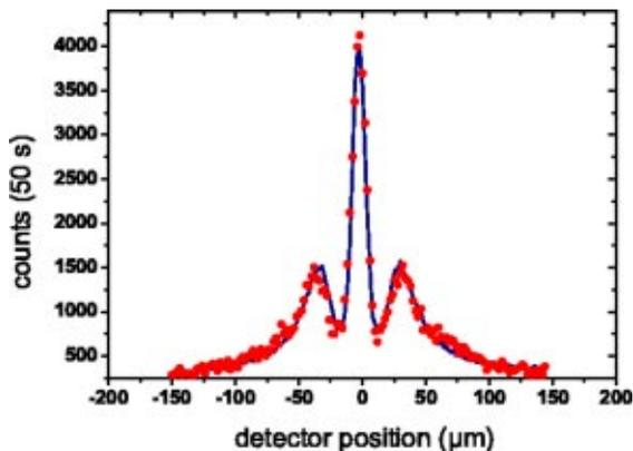
Fig. 6. Far-field diffraction of  $C_{60}$  using a thermal beam of  $\bar{v} = 200$  m/s with a velocity spread of  $\Delta v/v \sim 60\%$ . The absence of higher order interference fringes is due to the poor spectral coherence.
