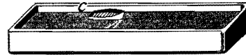
FIG. 14-35 Propulsion by Surface Tension. If the surface tension is different on a section of the periphery of the boat, there will be an unbalanced force on the boat.
