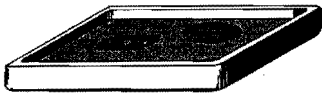
FIG. 14-34 Floating By Surface Tension Forces. Objects more dense than water float if they vary the surface area by a sufficiently large amount.
