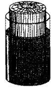
FIG. 14-16 Floating a Battleship in a Quart of Water. A very large block of wood will float in a very small amount of water, if the container and block are about the same volume.
