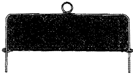
FIG. 14-28 Surface Tension. The stretched film tends to contract indicating that the energy decreases when the surface area decreases.
