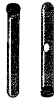
FIG. 14-18 No Gravitational Pressure in a Freely Falling System. Air bubbles will not rise while the system is freely falling.
