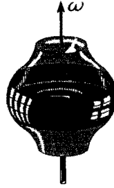
FIG. 14-20 Liquid Separator. A mixture of mercury and water separates with the mercury on the outside when the system is rotated.
