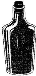
FIG. 14-17 Cartesian Diver. The vial can have its buoyant force varied by compressing the trapped air at its top.
