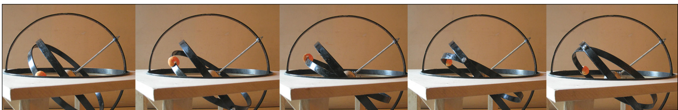
Fig. 5. Sequence of photographs of the armillary sphere with the Sun ball, both adjusted to show the positions of the Sun as seen by a resident of Albuquerque at different times of the day during the winter solstice.
